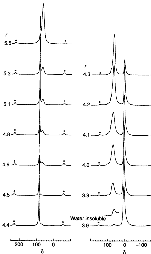
Fig. 1 ^{27}\text{Al} MAS NMR spectra of the sodium aluminates and aluminium hydroxides synthesized through acid hydrolysis for different values of r . The asterisks denote spinning side bands.
